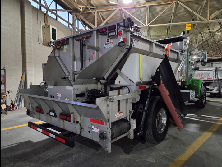
Duzmor w/ Cross Conveyor
