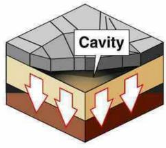
When temperatures rise, ground contracts; fractured and raised road surface is weakened by cavity below
