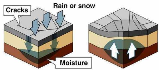
Rain, snow seeps into pavement, often through small cracks in road surface; saturates sub-base and soil below
