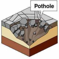
Damaged road surface cannot support weight of passing vehicles, breaks down, collapses into hollow space
