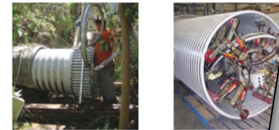
Figure 8: Spirally Wound Liner: Stationary (left) and Mobile (right) Winding Machines
