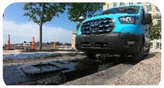
Energy transfer uses resonant induction between two coils.
