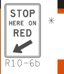
FOR USE WITH A RED/YELLOW LENS AFAD, ELIMINATE SIGN IF A RED/YELLOW LENS AFAD WITH A R10-6 SIGN MOUNTED TO THE DEVICE IS PROVIDED
