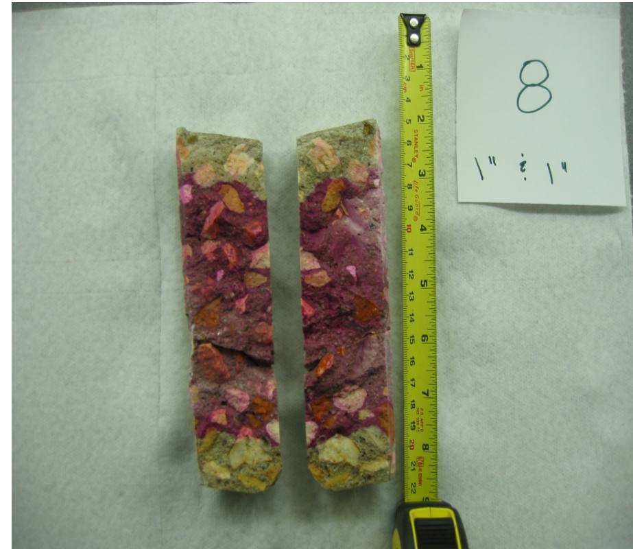
Carbonation Testing of Core Taken from Precast Double T Stem
