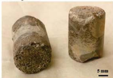
Example of cores were taken from bridge decks
