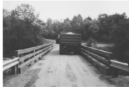
Figure 15—Transverse load test cases used for all spans: (top) load case 1, centered on roadway; (middle) load case 2, adjacent to upstream curb; (bottom) load case 3, adjacent to downstream curb.
