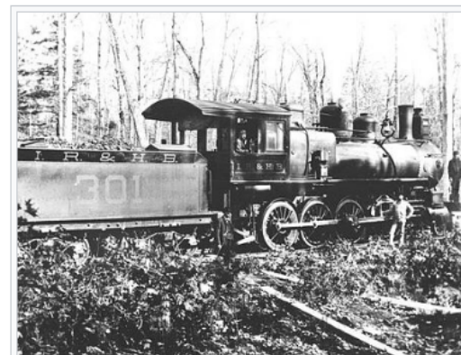
One of the two 4-8-0 locomotives owned by the IR&HB. They were later sold to the Algoma Central Railway .
