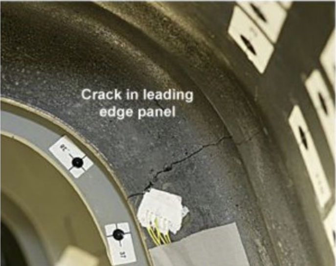
Damage done to wing RCC panels during foam impact tests
