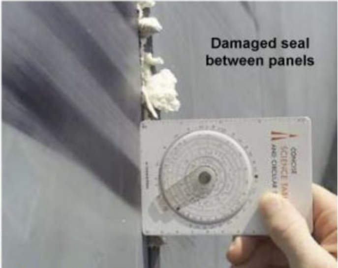
Damage done to wing RCC panels during foam impact tests
