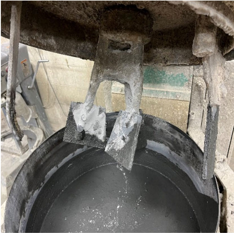
(a) F1 mixer (note side scrapers and high shear 'whirler' blades)
