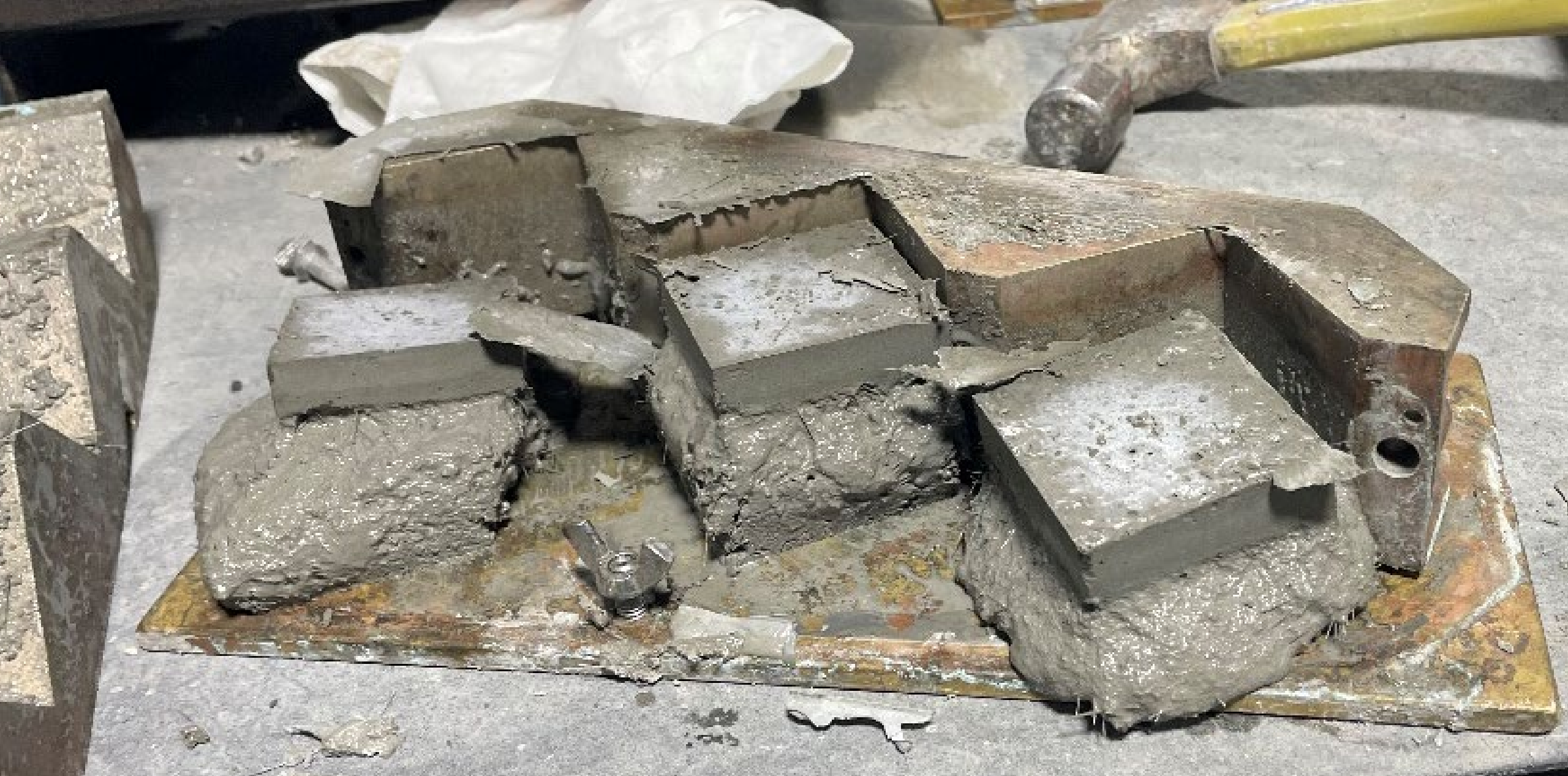
Curing in cold temperature (1 day)
