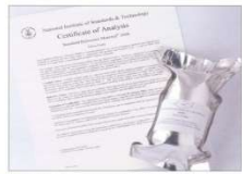
FIGURE 4.4. Silica fume Standard Reference Material (SRM 2850) available from the National Institute for Standards and Technology. Check either the Silica Fume Association or NIST web sites, as listed in the text, for instructions on how to order this material.
