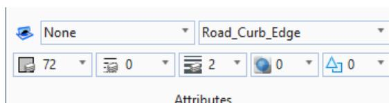
3. With the road centerlines highlighted, change the level to "Road\_Centerline".
