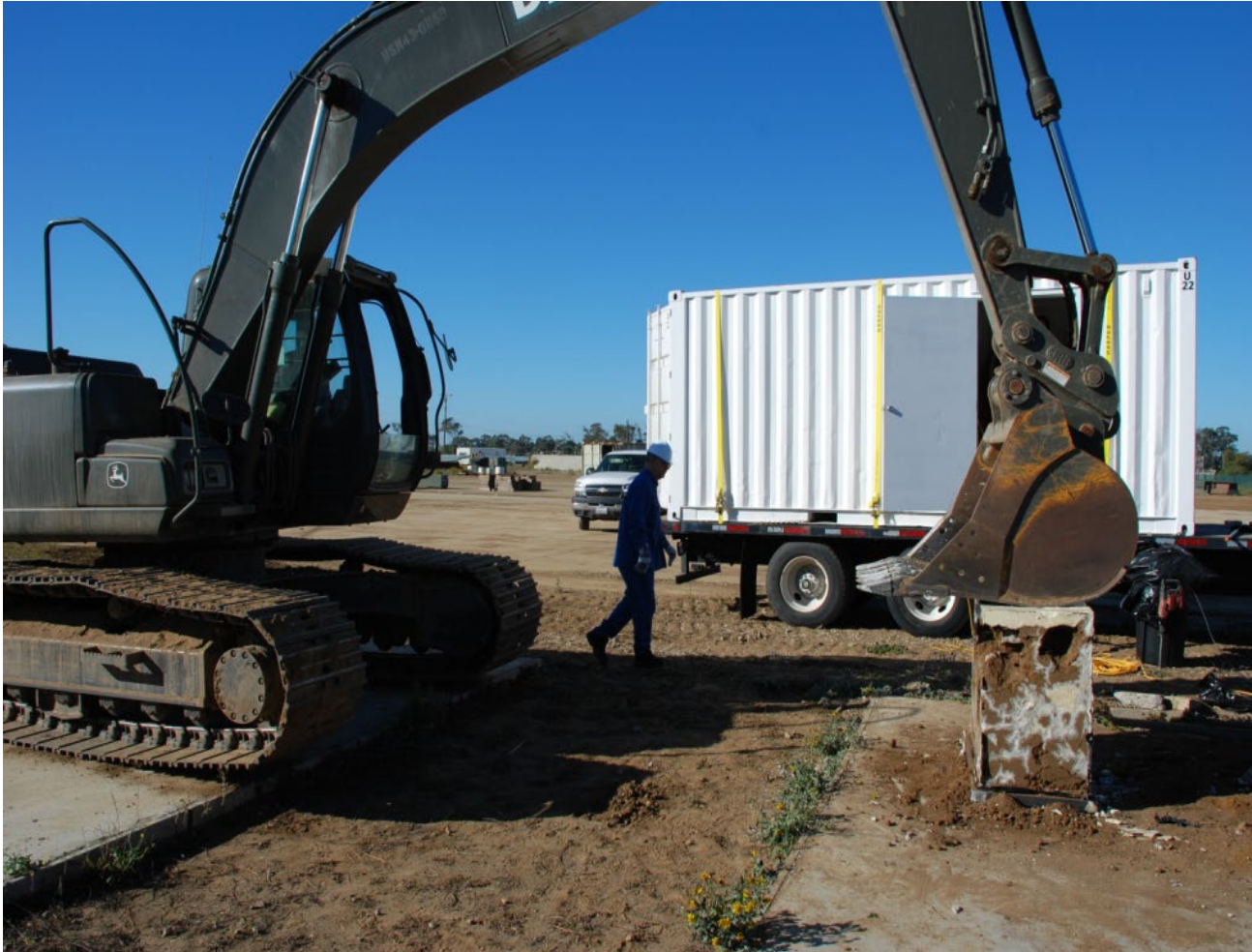
Vertical load applied using an excavator
