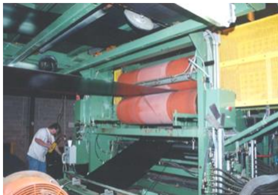
• Film lamination to steel strip.
