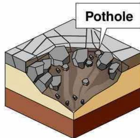
**4** Damaged road surface cannot support weight of passing vehicles, breaks down, collapses into hollow space
