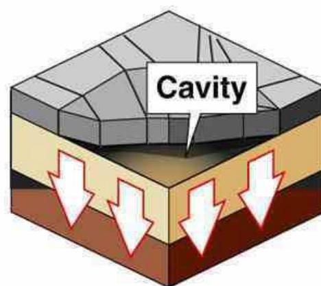
**3** When temperatures rise, ground contracts; fractured and raised road surface is weakened by cavity below
