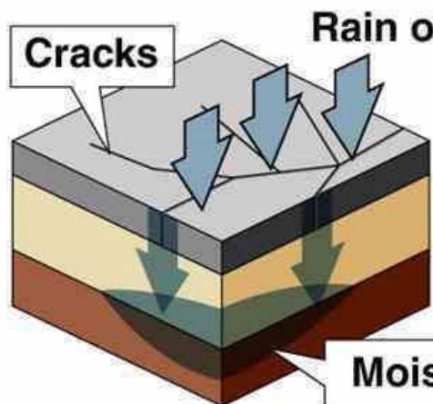
**1** Rain, snow seeps into pavement, often through small cracks in road surface; saturates sub-base and soil below
