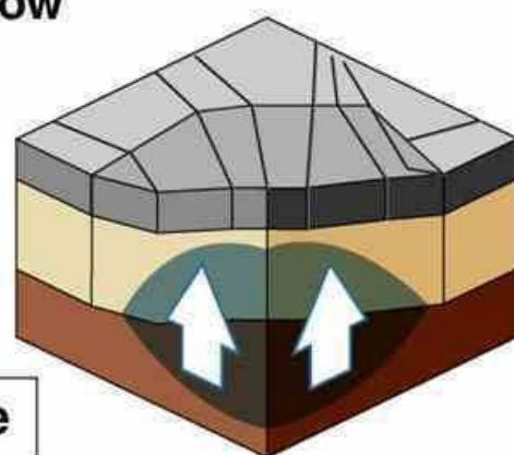
**2** During cold spells, moisture freezes and ground expands, pushing up, breaking road surface
