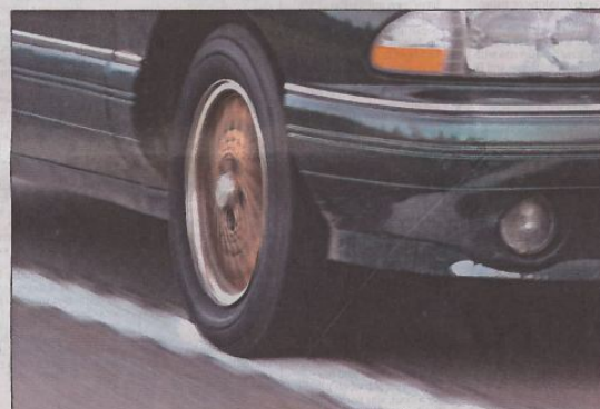
A car drives over a rumble stripe along County Road 4 on Thursday south of Biwabik. New highway safety guidelines required the strips to be moved 12 inches to ward the center of the road and onto the fog line, turning the old rumble "strip" into a rumble "stripe." Bob King / rking@duluthnews.com
