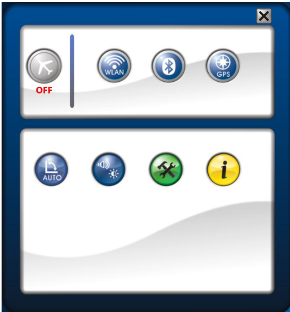
Figure 9 - Quickmenu Control Screen – if the GPS icon in the upper-right is blue the GPS is running
